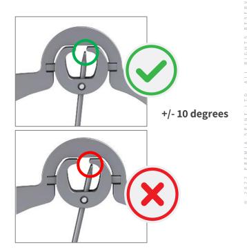
If outside of the notches, the screw must be repositioned
