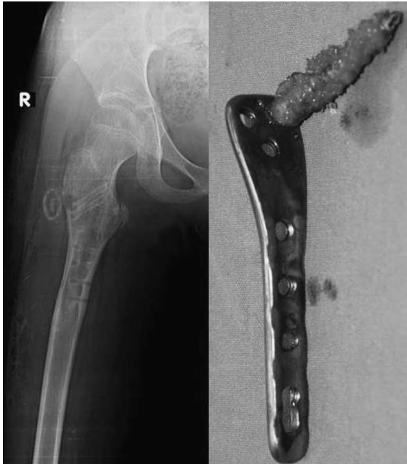
FIGURE 4. Intraoperative photograph shows cold welding and good bone-screw integration. Screw stripping occurred and the screw was removed with the plate. The bone was separated from its surroundings by forcibly dislodging the plate with an attached stripped screw. The detached part of femur was marked with red circle.
